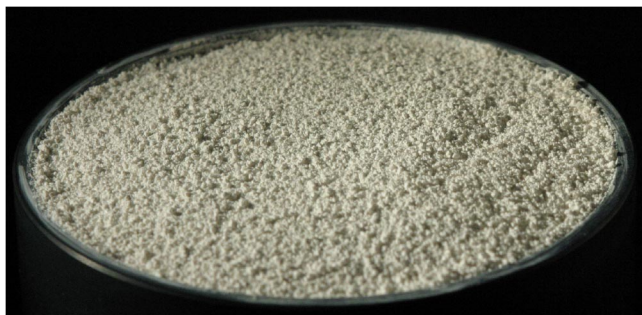
FIG. 4. A target prepared by sieving powder with a 0.5-mm mesh. The sieving results in a granular structure of the surface. The target diameter is 6 cm.
